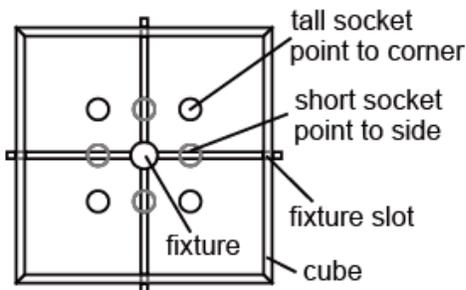
turn the cube(45 degree) to across middle flats, hang over the cube on the fixture slot.
