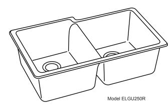
Undermount Installation Profile - 1/8" (3mm) Reveal
