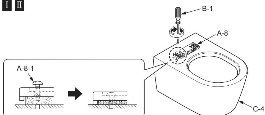
Failure to tighten screw A-8-1 completely will cause moving sideways of C-1.
