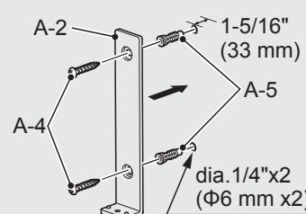
When mounting on a plaster board or tiled wall.
