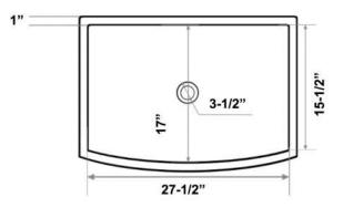
Dimensions of fixture are nominal and may vary within the range of tolerances established by ANSI Standard A112.19.2.2013 Dimensions and specifications subject to change without notice.
