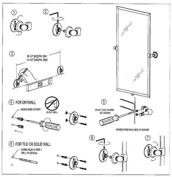
Tools needed: Pencil, Tape measure, Phillips Screwdriver, Drill and Level.
