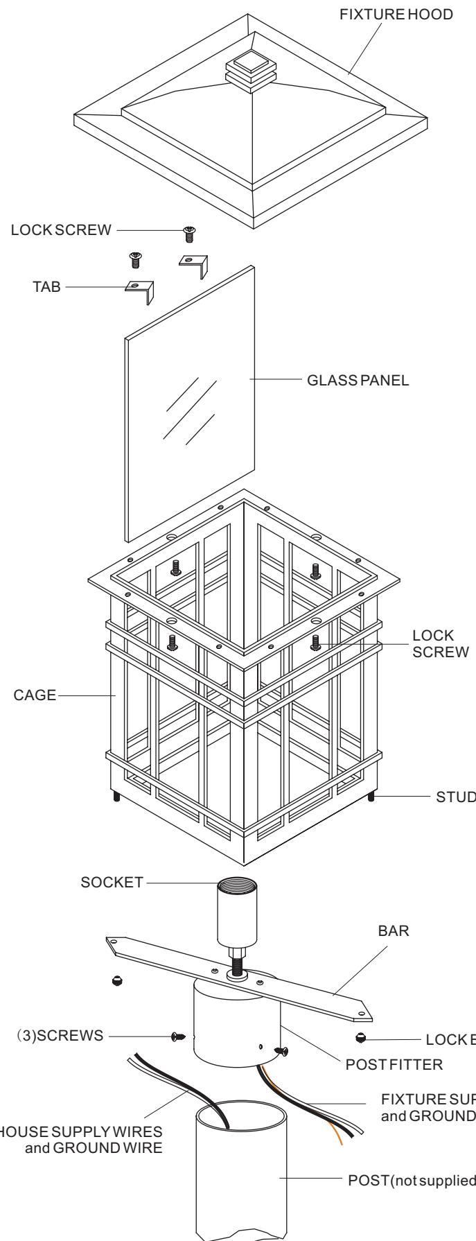
1. Before beginning the assembly/installation, carefully unpack and identify parts, referring to the illustration.
