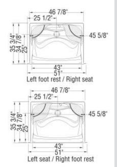
Flat surface for the installation of the valve 8-in. diameter All dimensions are approximate. Structure measurements must be verified against the unit to ensure proper fit.
