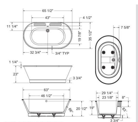
(()) :Recommended faucet area 2 sections of 16" (L) x 4" (W). Depth recommended for straight pipes 8".
