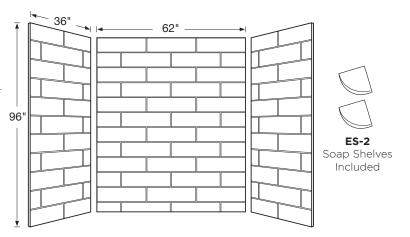
Designed to fit base areas 36" deep or smaller x 62" wide x 96" high or smaller (914 mm x 1575 mm x 2438 mm)
