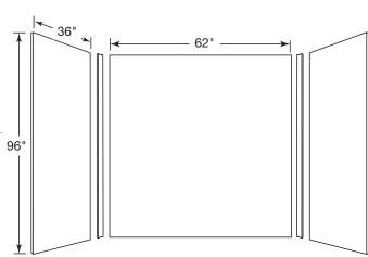
Designed to fit base areas 36" deep or smaller x 62" wide x 96" high or smaller (914 mm x 1575 mm x 2438 mm)
