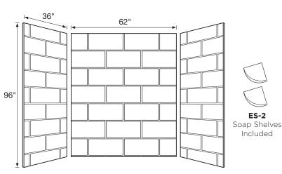
Designed to fit base areas 36" deep or smaller x 62" wide x 96" high or smaller (914 mm x 1575 mm x 2438 mm)
